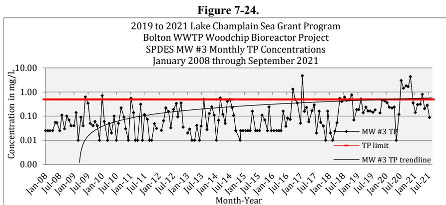
The reader should note that the *y-axis* in Figure 7-24 is in logarithm scale to accurately display the wide range of TP values measured for the SPDES permit TP samples collected from MW #3.
