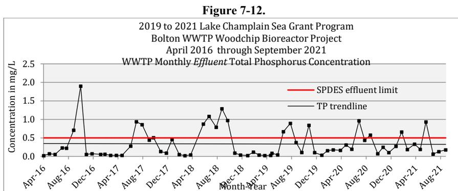
During the 66-month period shown in Figure 7-12, the TP concentration had an *average* of 0.34 (±0.39) mg P·L and there were 17 months when the concentration exceeded the SPDES permit effluent limitation of 0.50 mg P·L. Overall, however, there was a 10-fold reduction in TP concentration between *influent* and *effluent* streams with *influent* TP concentration having an *average* of 3.28 (±1.73) mg P·L.
