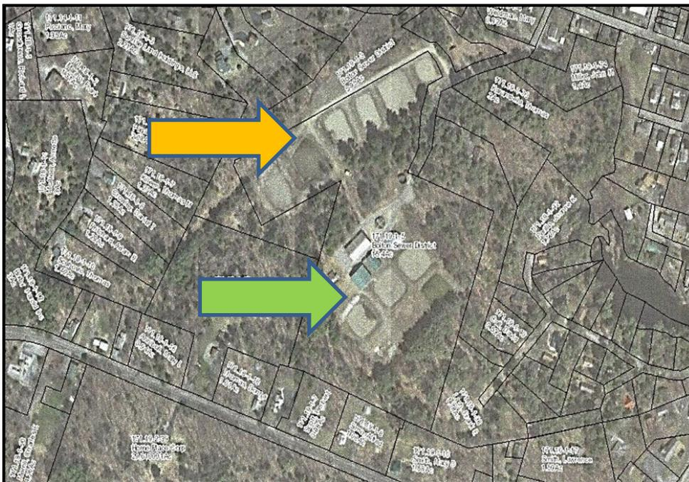
The configuration of the Bolton WWTP lot parcels is irregular. The treatment plant was constructed on the surface of a series of plateaus comprised of delta sand deposits, left by receding glaciers, in order to utilize the sand as an infiltration area for treated wastewater effluent. This is the same strategy used during the construction of the Village of Lake George Wastewater Treatment Plant (Sutherland and Navitsky 2015).
