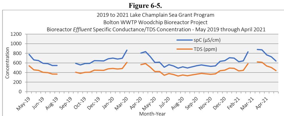
The spC concentrations measured for the bioreactor *influent* ranged from 491.1 to 1088  $\mu\text{S}\cdot\text{cm}$  @ 25C while bioreactor *effluent* concentrations during the study ranged from 490 to 879.6  $\mu\text{S}\cdot\text{cm}$  @ 25C. The *mean* spC concentration for the bioreactor *influent* and *effluent* during the study is presented in Table 6-2; values were 671.4 and 640.4  $\mu\text{S}\cdot\text{cm}$  @ 25C, respectively.
