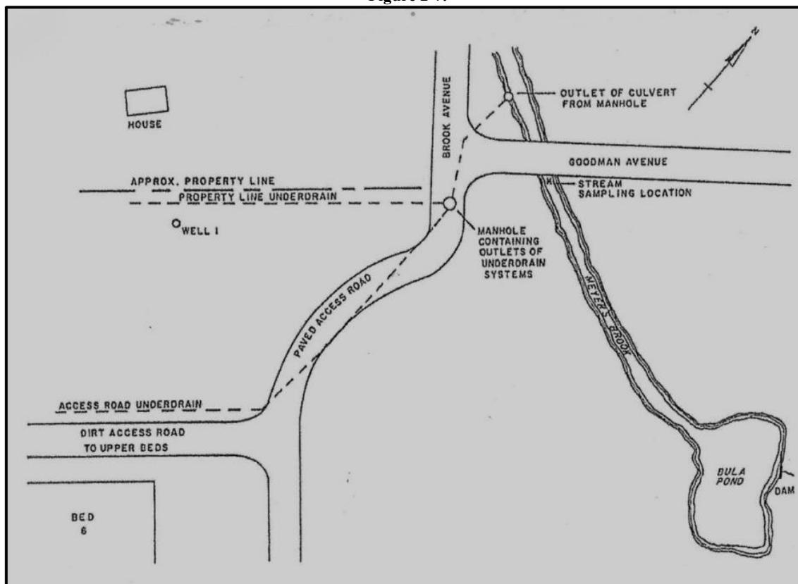
The dye was added to Bed #8 on May 25<sup>th</sup> and was detected on May 30<sup>th</sup> at (1) the outlet of the property line underdrain, (2) the outlet of the culvert that drains into Stewart Brook, and (3) in Stewart Brook. The dye was detected at the Stewart Pond dam/spillway on June 2<sup>nd</sup>. No dye was detected in Monitoring Well #1 or the access road underdrain.
