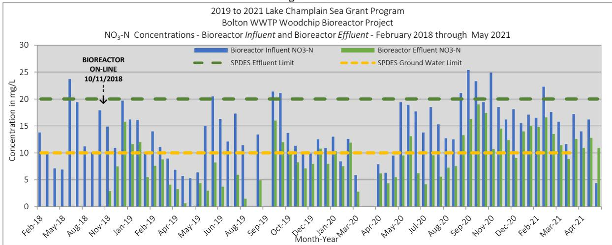
The following graph, Figure 6-17, summarizes the percent removal of  $\text{NO}_3\text{-N}$  from the Bolton WWTP effluent that enters the bioreactor:
