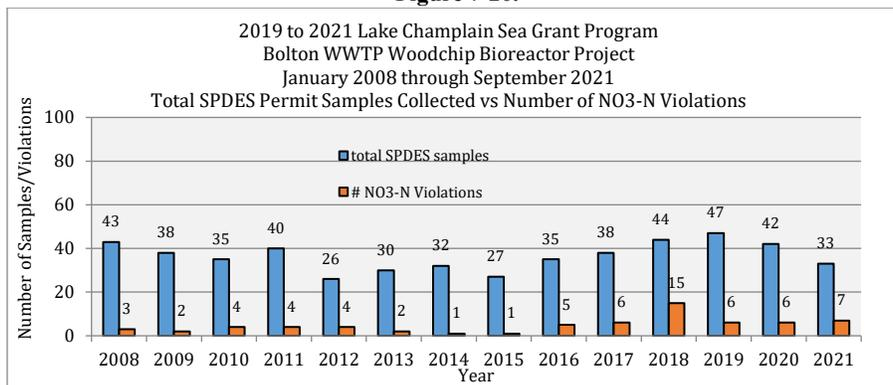
Once again, it is interesting to attribute the decline in NO<sub>3</sub>-N violations from 2019 through September 2021 to the installation of the woodchip bioreactor in the area of the upper sand beds and the ability of this unit processor to reduce the NO<sub>3</sub>-N concentrations leaving the Bolton facility in wastewater effluent. There will be more evidence and discussion related to this topic later.
