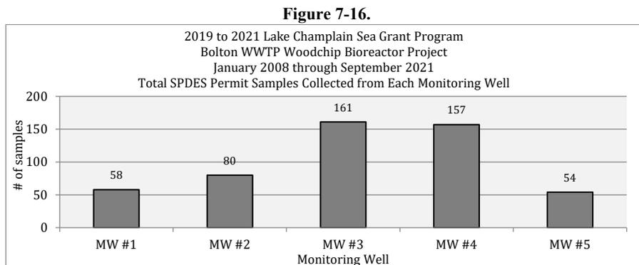
Based upon the total number of samples collected from the SPDES permit MWs shown in Figure 7-16, MWs #1, #2 and #5 appear unable to provide regular samples for SPDES testing. There are several factors that affect the data shown in Figure 7-16, however, that should be considered:
