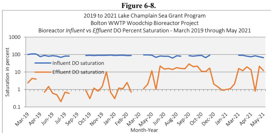
A comparison of the *influent* and *effluent* **DO** concentrations for the bi-weekly sampling is presented in Figure 6-9.
