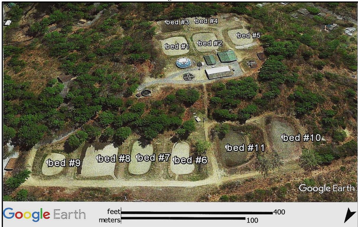
Sand beds #1 and #3 are dosed with effluent through a center-feed discharge device consisting of an upright 20.3 cm (8 inch) PVC pipe surrounded by a 1.2 m (4 ft) square concrete splash pad. The other lower beds are dosed through a pipe that enters one side of the bed. All plant effluent is dosed to a single bed at a time and the bed dosing sequence is random, chosen by the operator, and recorded in a daily logbook.
