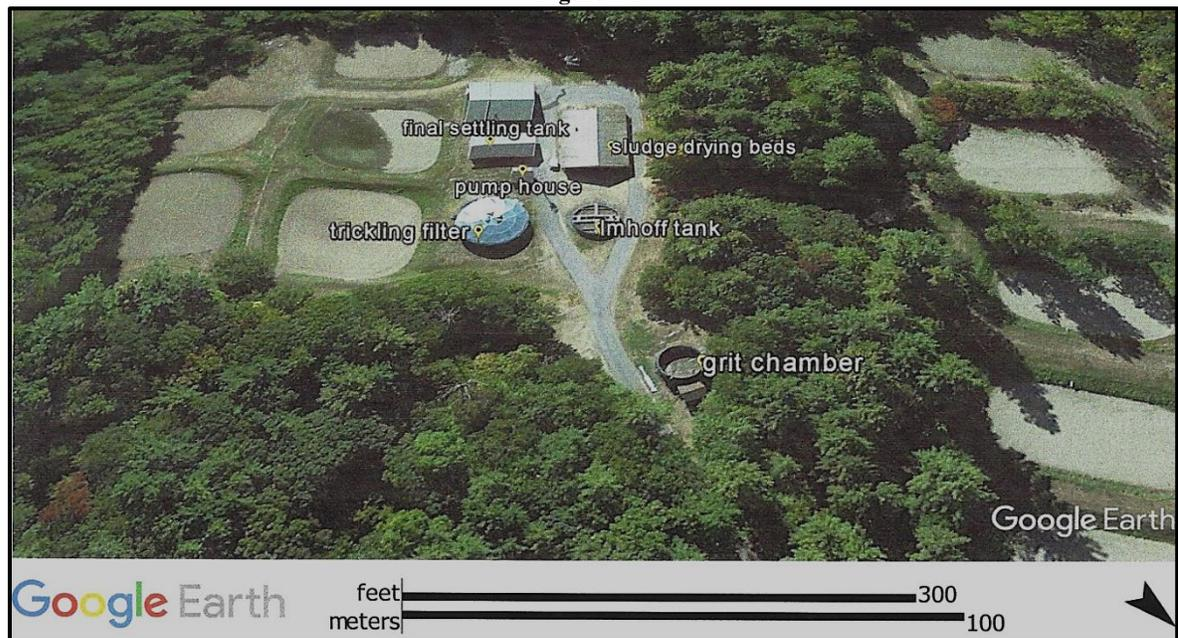
The primary effluent is fed to a 16.7 m (55 ft) diameter rotary distributor trickling filter and then to a mechanically cleaned rectangular final settling tank. The unchlorinated plant effluent is discharged to sand filter beds on site. Digestion of the primary and return secondary sludge is accomplished in the lower chamber of the Imhoff tank.
