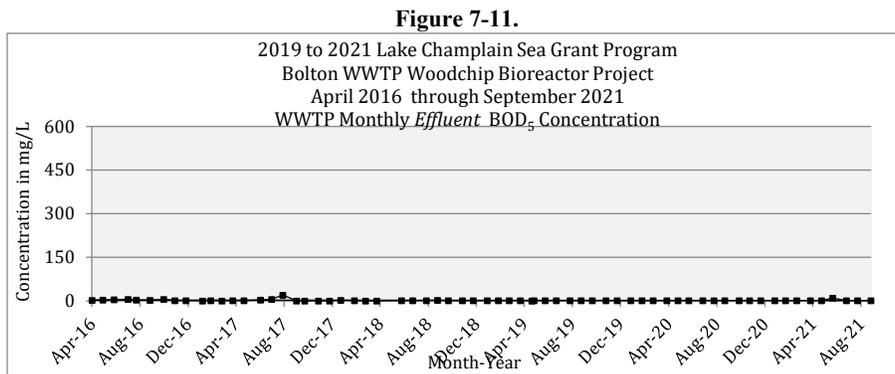
As with TSS described above, a comparison of Figures 7-6 and 7-11 shows that all BOD<sub>5</sub> is removed from wastewater processed through the Bolton facility before being discharged as *effluent* to the local ground water.
