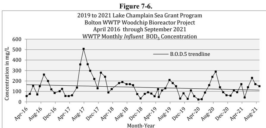
In general, BOD<sub>5</sub> concentrations varied from about 20 to 300 mg BOD<sub>5</sub>·L except for a period during 2017, from July through November, when *average* values all were above 200 mg BOD<sub>5</sub>·L (Figure 7-6). Since that time, there only were three results more than 200 mg TSS·L and, as the trendline in Figure 7-6 shows, there has been a steady decline in the *influent* concentration of TSS.
