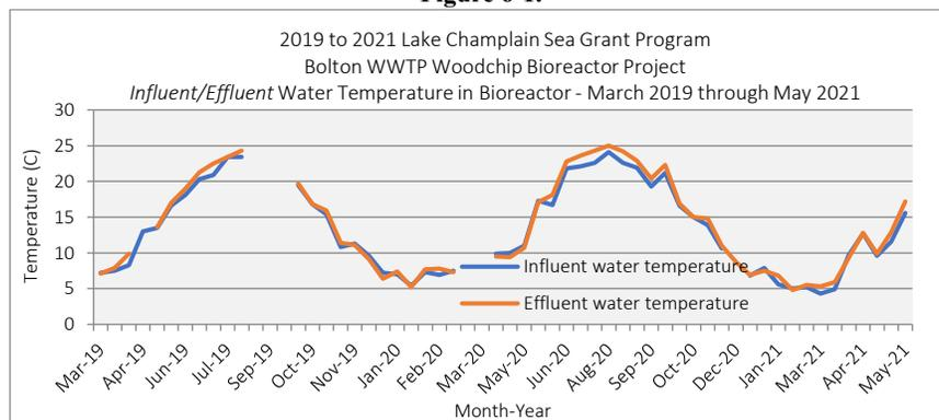
The pattern of *influent* and *effluent* temperature in the woodchip bioreactor mirrors the ambient outside temperature which is higher in the summer months and lower in the winter months because the majority of the tanks in the WWTP process are either exposed directly to the outside or in unheated shelters.
