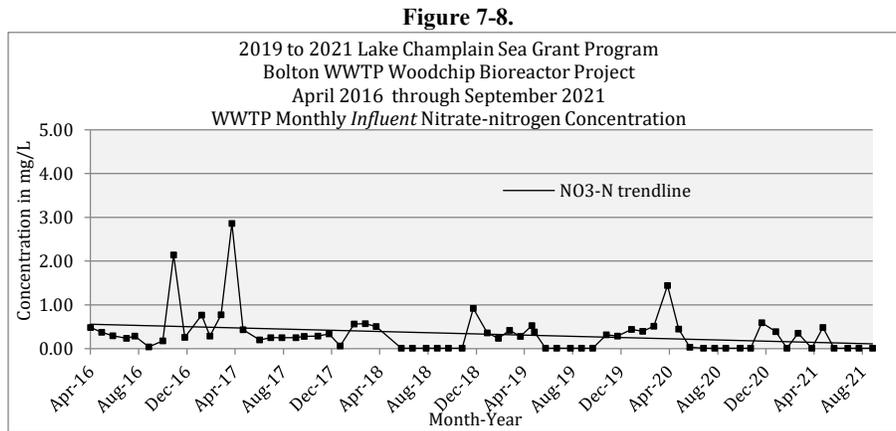
In contrast to the other wastewater influent parameters discussed in this section, the peaks in NO<sub>3</sub>-N concentrations corresponded to the colder months of the year while the lower concentrations occurred during the late spring and summer months (Figure 7-8).
