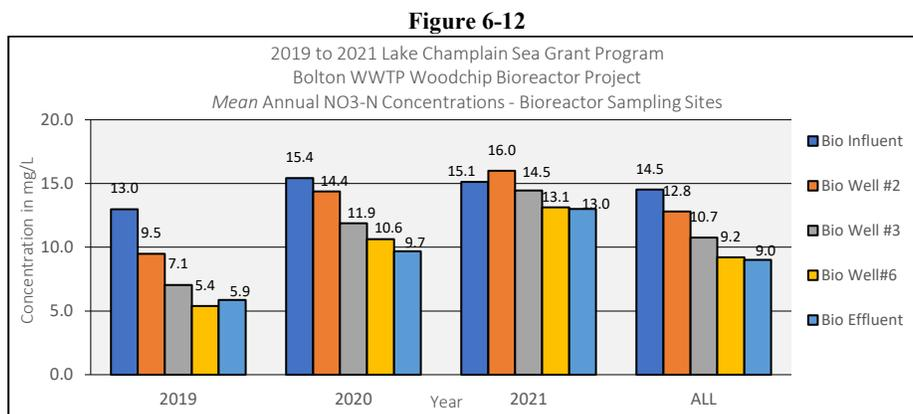
The *mean* NO<sub>3</sub>-N concentration among the bioreactor sampling sites varied from 5.4 (Bio Well #6 – 2019) to 16.0 mg N·L (Bio Well #2 – 2021). The general trend for NO<sub>3</sub>-N concentration in the series of bioreactor well sites was a decrease from *influent* to *effluent*, indicating successful denitrification in the bioreactor.
