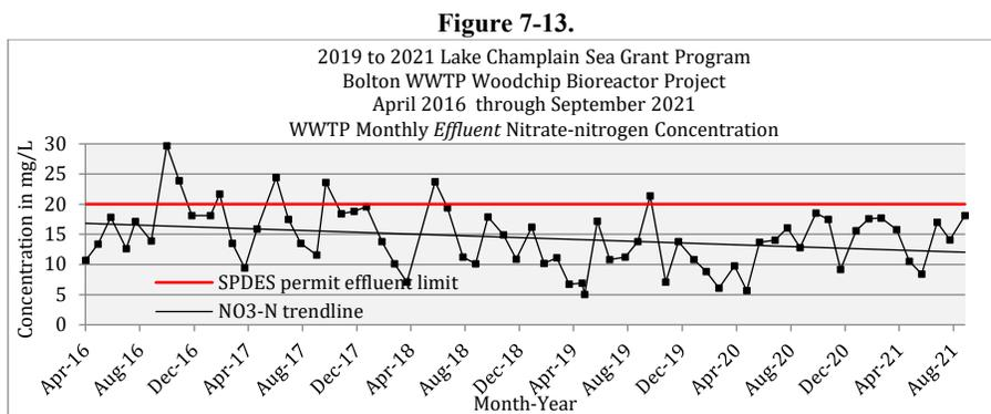
The facility *effluent* NO<sub>3</sub>-N concentrations discharged to the sand beds were more than 20 mg N·L on only 7 occasions during the 66-month period, and the NO<sub>3</sub>-N trendline in Figure 7-13 clearly shows that *effluent* concentrations have been declining during the entire period.
