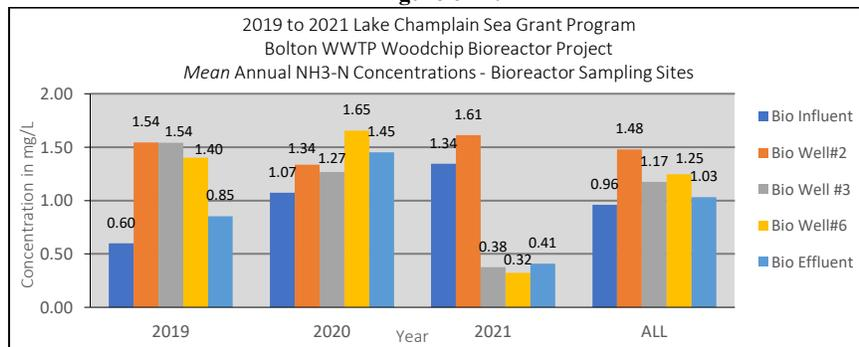
The bioreactor sampling site **NH<sub>3</sub>-N** concentrations varied from 0.32 mg N·L (Bio Well #6 – 2021) to 1.65 mg N·L (Bio Well #6 – 2020). There was no trend apparent for **NH<sub>3</sub>-N** in the series of bioreactor sample sites during the study.
