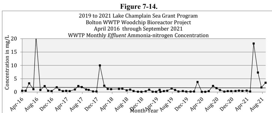
As shown in the figure above, the trendline for the ammonia-nitrogen concentration since April 2016 has been flat, indicating that no apparent increasing or decreasing trend is occurring. There were, however, three (3) months since June 2021 when ammonia-nitrogen concentrations in *effluent* leaving the facility were in excess of 2.0 mg N·L (see Figure 7-14).
