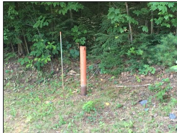
A third monitoring well (#4) is located up-gradient of any ground water movement away from the upper-level sand beds (see Figure 5-2) and was selected as a site that would provide water quality characteristics
