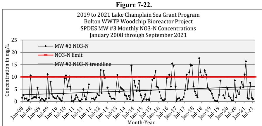
Although most of the reported concentrations are below the threshold of 10 mg N·L, the NO<sub>3</sub>-N trendline in Figure 7-22 predicts that increasingly more samples will be reported as SPDES permit violations in the future when looking at the data from January 2008 through September 2021.
