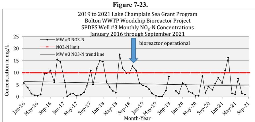
From January 2016 through September 2018, there were a total of nine (9) NO<sub>3</sub>-N concentration violations measured in MW #3, with a similar recurring pattern of concentration exhibited during each annual cycle. Beginning in October 2018, a noticeable decrease in the pattern of NO<sub>3</sub>-N concentrations occurred, and only two (2) NO<sub>3</sub>-N monthly concentrations exceeded the SPDES permit limit through the end of September 2021.
