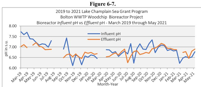
All of the recorded values for pH were above pH 6.0 for the *influent* and *effluent* with an *influent* range from 6.11 to 7.73 and the *effluent* from 6.21 to 7.21. The average pH is shown in Table 6-2 for the bioreactor *influent* and *effluent* and were 6.90 and 6.78 s.u., respectively. It is stated that the optimum pH values for denitrification are between 7.0 and 8.5 (Dangcong et al. 2004).
