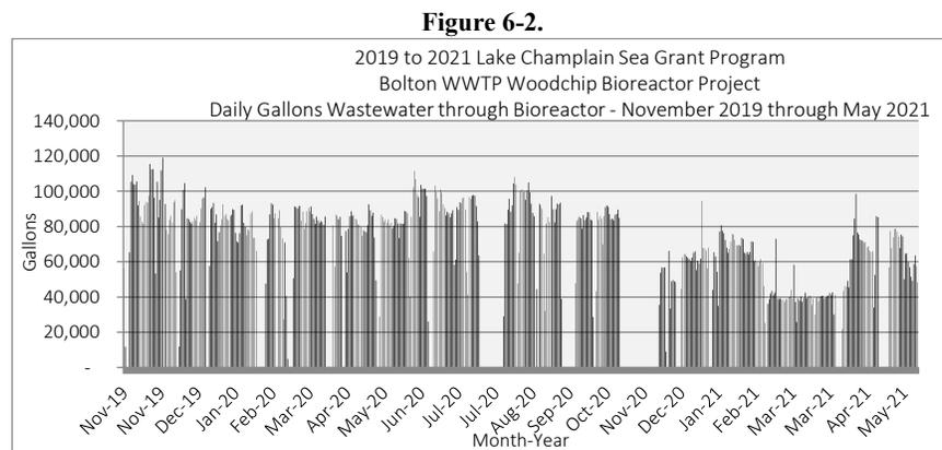
This flow reduction was intended operationally to optimize *denitrification* through greater retention time during a period when higher than typical influent nitrate concentrations and colder wastewater temperatures were observed.
